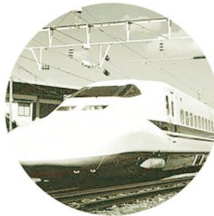
Aluminum extrusions are used for the exteriors of Nozomi 700 series shinkansen cars
